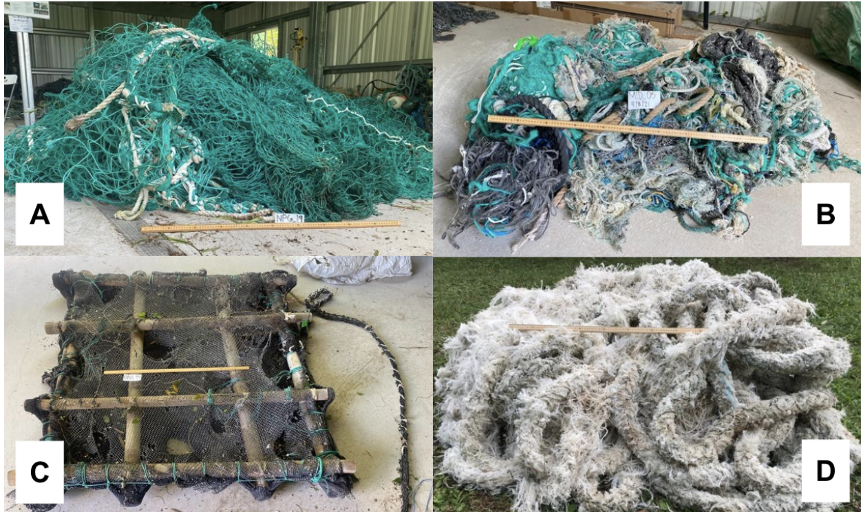
Figure 2.1. The four primary DFG categories that were encountered, sampled and analyzed using the methods described in this document include distinct net (A), conglomerate (B), drifting fish aggregating device (C), and line (D) (See Glossary).
