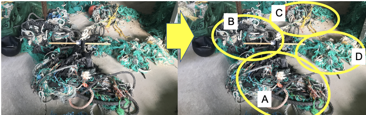
Figure 2.9. This figure shows a DFG event that was sampled using the Hybrid method. The event was spread apart into sections, as shown on the right.
