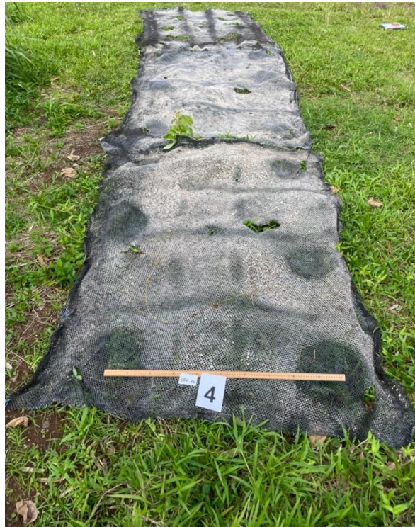
Figure 2.15. The black netting that wraps a dFAD raft laid out to measure.
