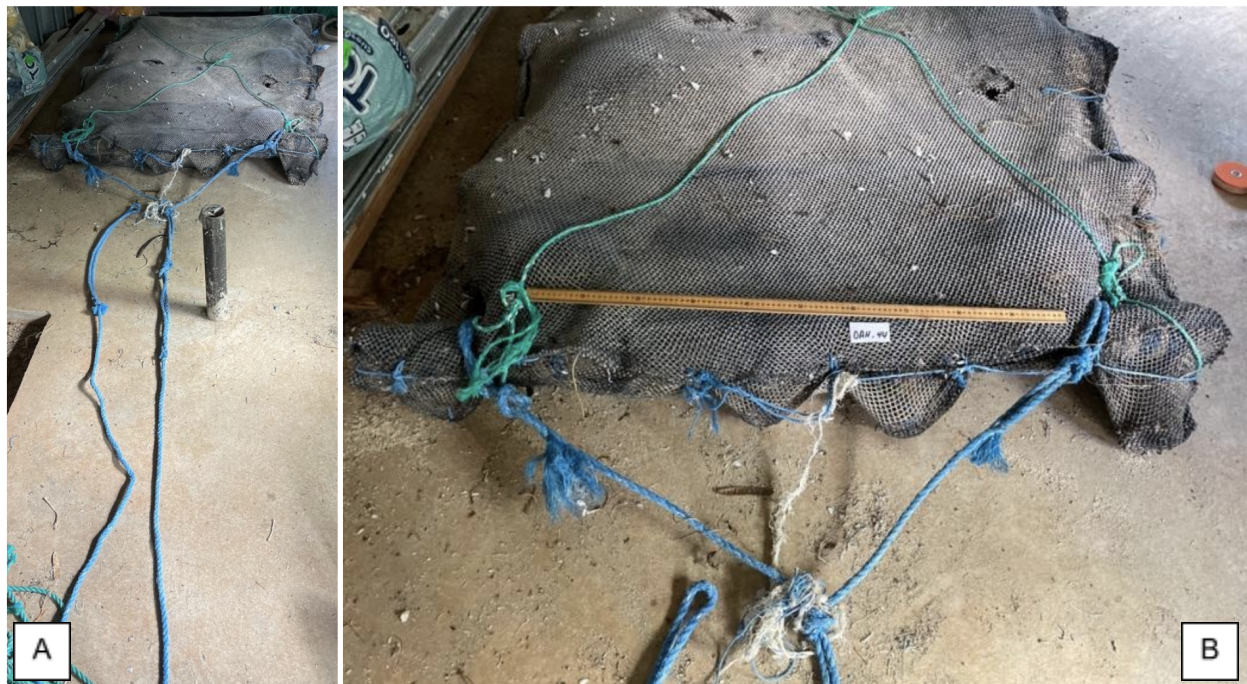
Figure 2.12. Drifting fish aggregating device (dFAD) from the tropical tuna purse seine fishery. A) The blue line makes a bridal and attaches to the SAT buoy that is stretched out to measure the length. B) Close-up of the blue bridal line and green lines created as a pick point to lift the dFAD.
