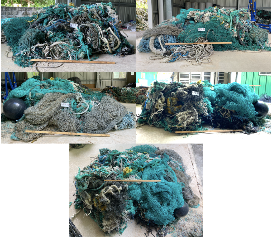
Figure 2.4. Example of the standardized five photos of a conglomerate DFG event. The bottom image is a top view of the DFG event. A meterstick scale bar and DFG event ID tag are in each photo.
